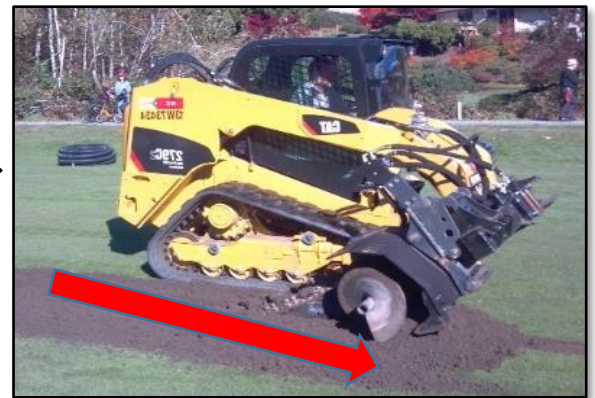
SideTool SideTrencher Coupler folded out to place trencher to the side
